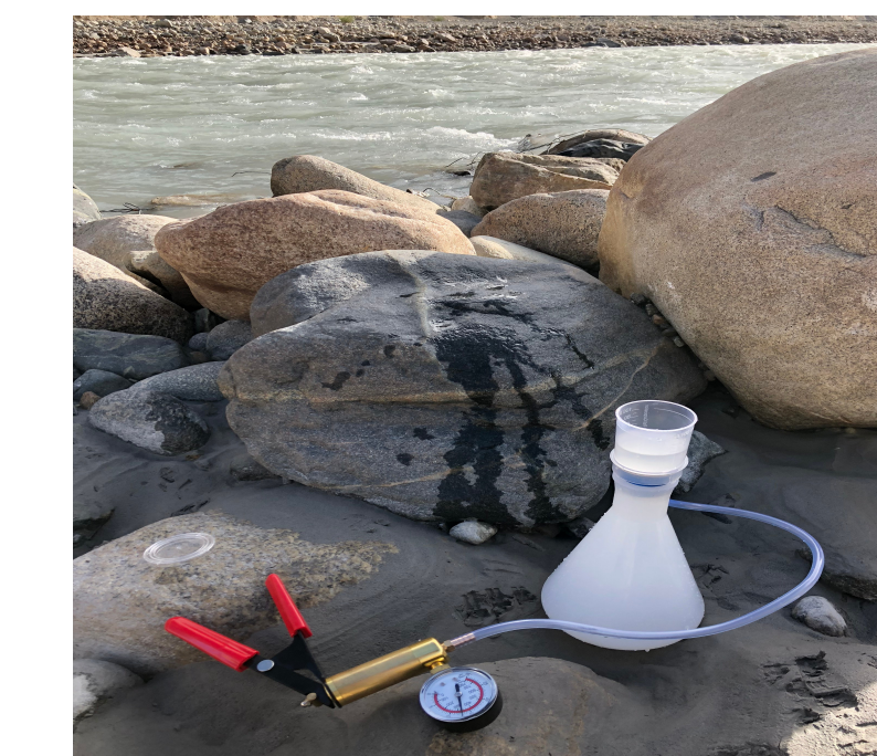
Filtering water sample using vacuum pump
