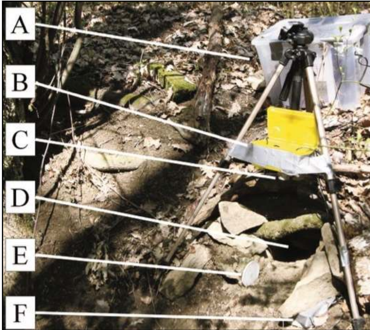
Camera Trap with Active Infrared Sensor AIR
